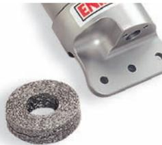
**Wire mesh material can be manufactured** in a multitude of shapes and sizes to accommodate your specific application. When exercised, the wire mesh damping elements convert input energy to heat. Friction is created when knitted or woven stainless steel wire strands are displaced relative to one another. Knitted metals have inherent resiliency and provide high-damping characteristics and non-linear spring rates.
