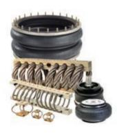
Wire Rope Isolators are helical wound cable isolation mounts that offer multi-axis, maintenance-free shock and vibration isolation within a wide operating temperature range. Comprised of stainless steel cable threaded through aluminum alloy retaining bars, Wire Rope Isolators are not only rugged, but versatile for any application, our various models of Air Springs and custom elastomeric products offer the versatility to control motion, noise and vibration in a variety of industrial applications.
